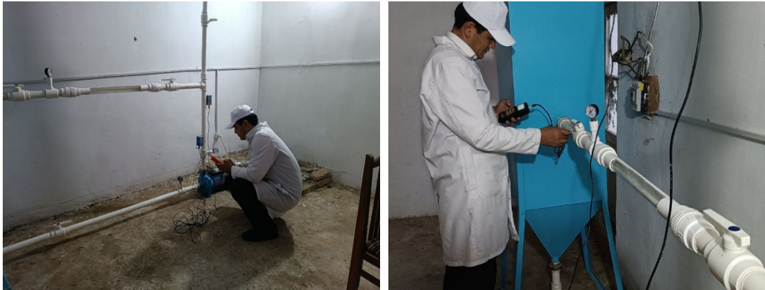
Figure 3. Application of flowmeter and ultrasonic flow measuring device in laboratory conditions.
