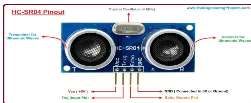
2-rasm. HC-SR04 tovush sensori.
