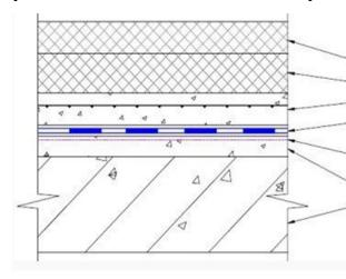
Figure 1. The top layer of asphalt concrete The lower layer of asphalt concrete Protective layer with reinforcement TEHNOELASTMOST B Polymer-bitumen TechnoNIKOL #3 Leveling layer Reinforced concrete slab
