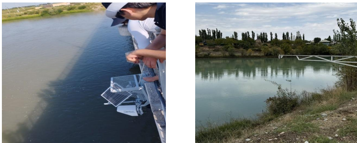
Figure 2. Automated water metering devices installed in Namangan region
