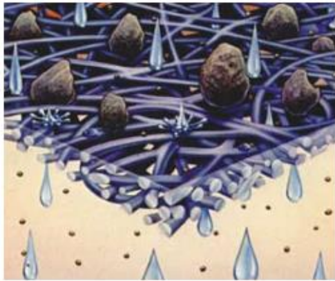
Figure 1. Water permeability of geotextile Figure 2. Location of geotextile on the floor
