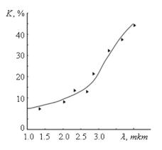
Fig 2. The dependence of the light reflection coefficient on the light wave length for the 200 Å thickness film hence the absorption coefficient sharply decreases. Apparently, that results in some increasing of the light reflection coefficient.
