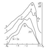
Fig 1. The photoelectrons spectra for the Si (111) and  $CoSi_2$  films (d=200 Å) measured at  $hv=10.8 \ eV$ .
