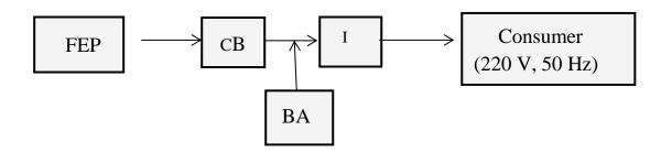
FEP photoelectric plate; CB-control block; RB-rechargeable battery; I-inverter.
