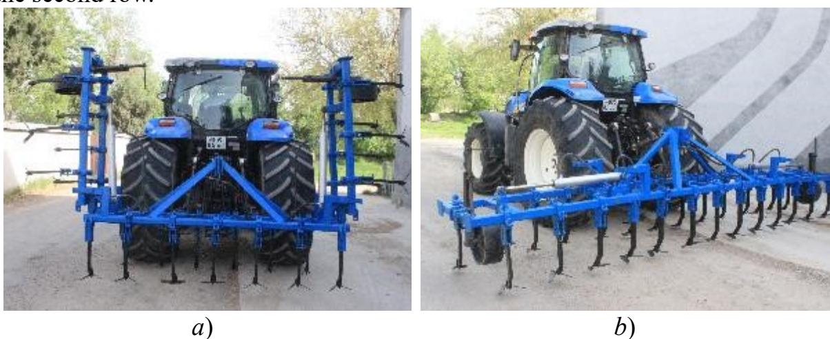
Figure 2. Views of the experimental model of the wide-coverage chisel cultivator in transport (a) and working (b) positions
