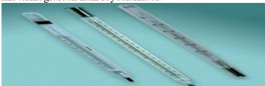
1- rasm. TM-1 - rusumli meteorologik termometr
