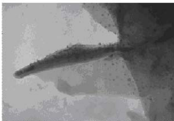
Rice. 5. Microphotograph obtained using TEM and reflecting the moment of folding of a nanofilm with small formations of graphene and nickel nanocrystals.
