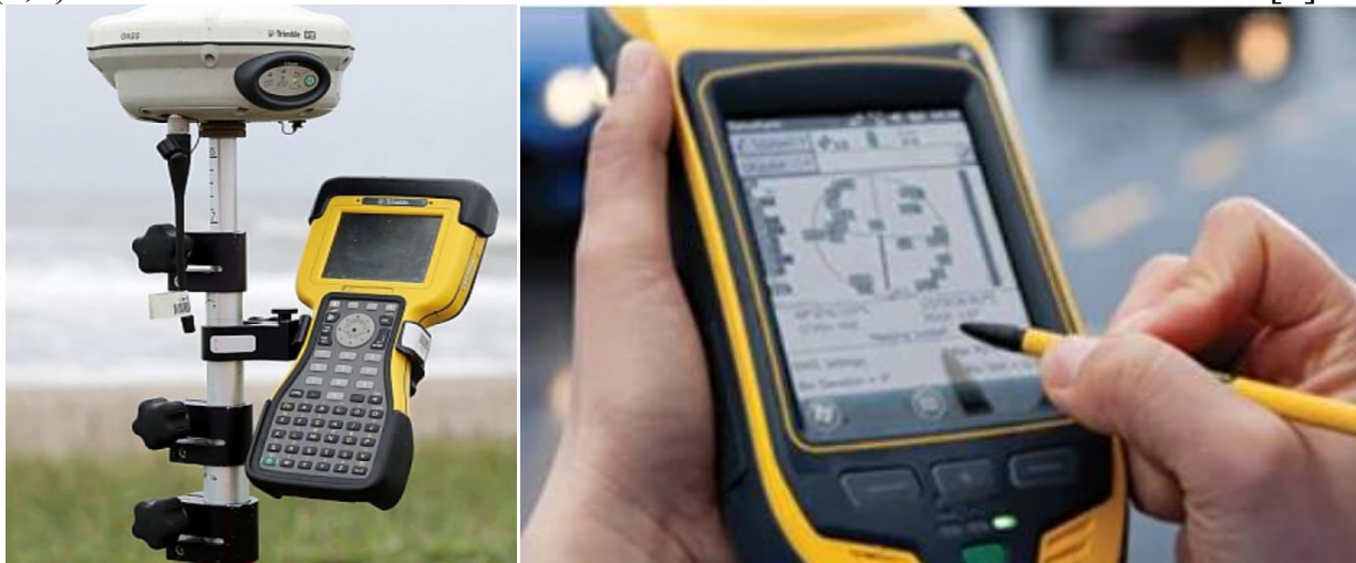
Figure 3. GPS receivers. Source: https://geo-teo.ru/stati/gps-priyomnik-geodezicheskij/ va https://www.trimble.com/en/solutions/technologies/positioning
