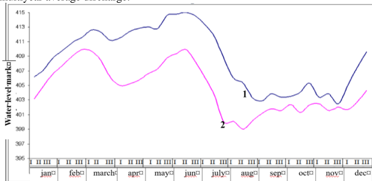
Figure 2.1 Queuing chart for effective reservoir filling and emptying.
