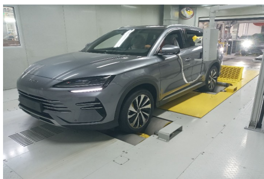
Figure 1. Test layout of the braking system of the BYD SONG PLUS CHAMPION electric vehicle.
