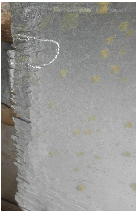
Fig.1. Wear of the working blade after 1800 hours of operation.
