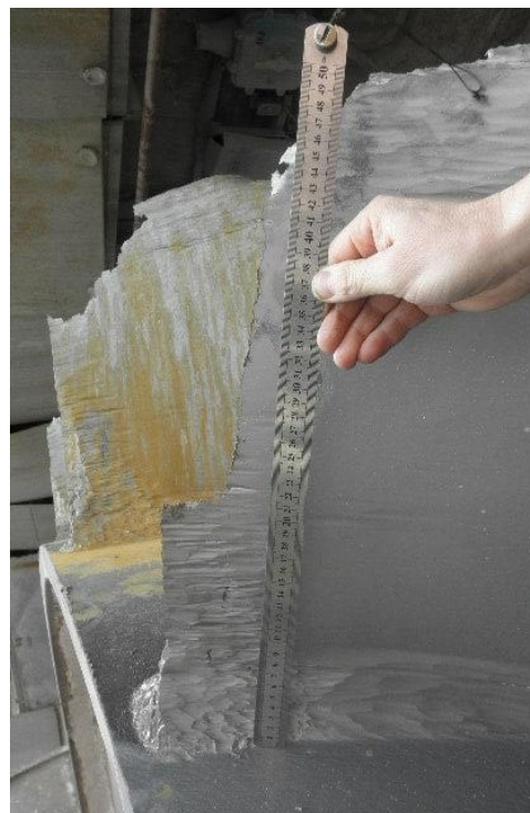
Fig.2. Wear of the working blade after 4200 hours of operation.
