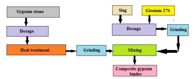
Fig. 1. Obtaining a composite gypsum binder according to the first method
